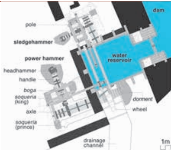
Ground plan of the power hammer and th sledgehammer from the Rossell forge (ARH).
